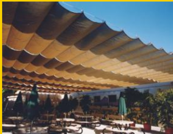
Retractable Slide-on-Wire canopy for covering large open areas. Fabric tarp is suspended from stainless steel cables that ride on nylon pulleys.
