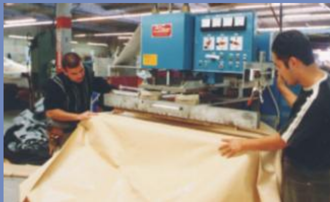
Radio Frequency fabric welding of 18 oz. vinyl for clean room curtains.
