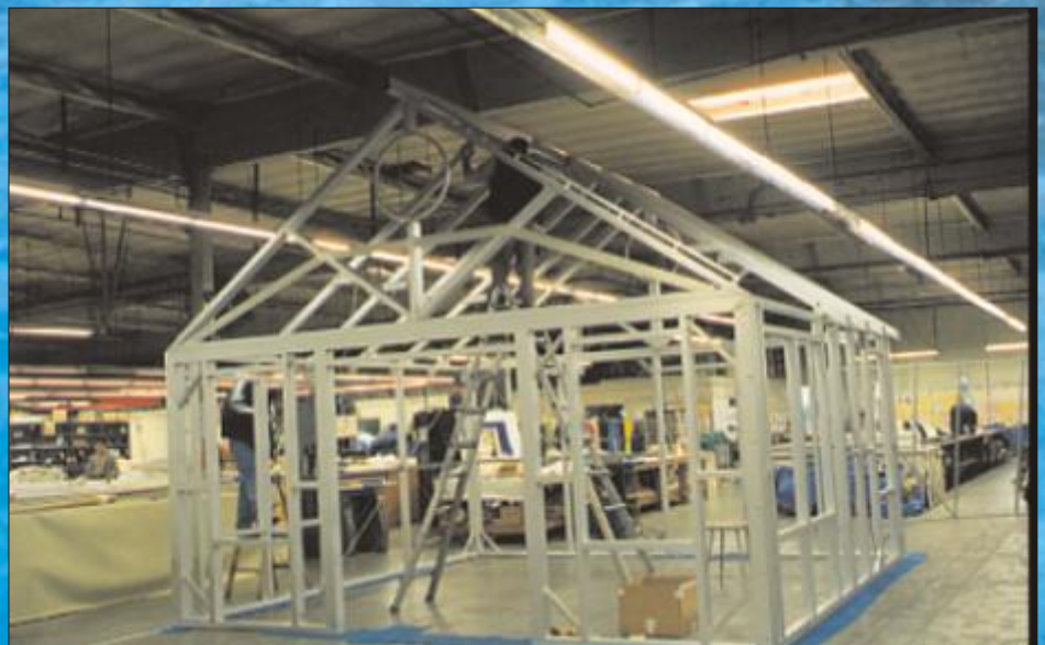
Frames are designed and engineered to meet the requirements of each customer and project. The Eco-Tent framework shown here is anodized aluminum and designed for 110 m.p.h. wind loads. Walls and components are prefabricated to reduce assembly and installation costs.
